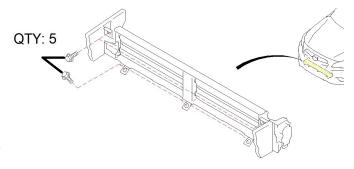
Step 3. Remove the temperature sensor from the Passenger side of the Active Shutter Assembly by pinching the upper and lower sides of the clip built into the sensor from the backside of the assembly. This sensor needs to be re-connected and ziptied somewhere inside the lower grille area but not
