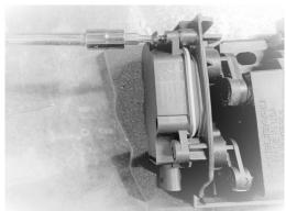
Step 5. Install the ASE assembly onto the Active Shutter Motor, if your Active Shutter assembly has previously been removed or damaged you may need to use the ASE Assembly to rotate it slightly back to the correct start position, the motor puts up some resistance but with enough force it can be moved. Looking at the motor from the side with the internal splines, the "arm" on the ASE needs to be all the way counter clockwise in the radial slot, see photos below.
