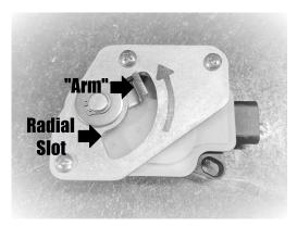
Step 6. Now that the motor is in the correct position, place a nylon spacer in between the motor and the ASE at each screw position and install the #8 screws through all three components and secure with the Nyloc nuts, use the #2 Phillips Screwdriver and the 11/32" socket to tighten everything, the torque spec for bolts this small is ~20 Inch/lbs, that's \*\*\*\*\*\*\*\*INCH POUNDS\*\*\*\*\*\*\*\*\* not ft/lbs, over tightening may break the mounting holes on the motor.
