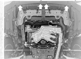
3. Thread two of the M8x20mm JIS Flange bolts into the rearward location where you removed two of the 12mm headed bolts that held the "H-shaped" black steel longitudinal bracket. Thread the bolts in about 3 turns.
