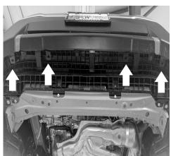
3. Thread two of the M8x20mm JIS Flange bolts into the rearward location where you removed two of the 12mm headed bolts that held the stock splash shield onto the car. Thread the bolts in about 3 turns.
