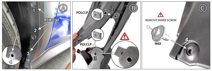
**FIGURE D/E** Adhere SMF29-1 **directly onto fender liner** of mount 2. Position BMF92-FRT bracket against flap mount 3. Curved section of bracket points to the ground. Install 1SS into BMF92-FRT mount 3. Use 1SS and SMWASH into mount 2. Position .5SP spacer **behind** flap mount 4 over INS2. Install 1.5SS & SMWASH through flap, .5SP and into INS2. Do not fully tighten.
