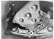
3. Remove the two 17mm Headed nuts holding the front of the differential to the differential mount.
