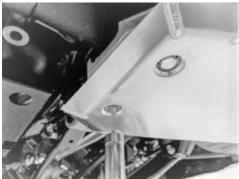
5. Install the QTY:3 M6 countersunk bolts up through the Skidplate and tighten them with the 10mm headed nuts (~10ftlbs)
