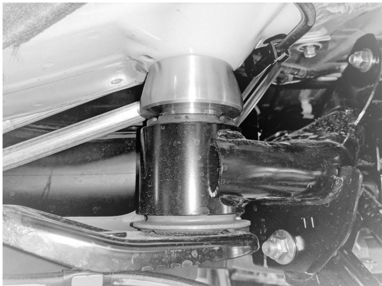
PRSS Main Spacer Installed:
