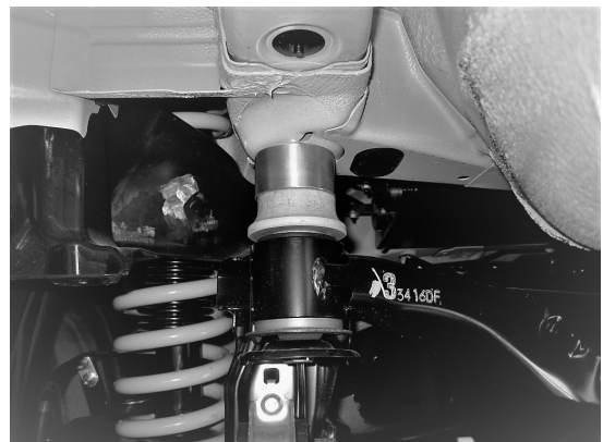
Installed subframe spacers:
