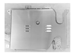
2. Remove the 4 x 19mm headed bolts indicated in the photo, the 2 rear bolts won't be re-used in the installation but the front 2 bolts will, so keep them handy.
