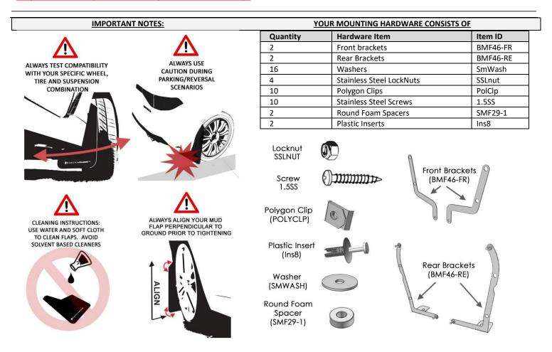
Recommended tools: Offset, ratcheting or stubby Phillips screwdriver, small flat head screwdriver, 7/16" wrench.
