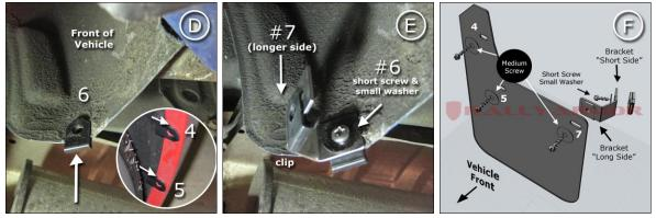
Confirm the edge of the flap is perpendicular to the ground. If needed, make slight adjustments by shifting the upper or lower portions of the flap. Check each incremental adjustment by walking away from the vehicle and looking at the mud flap directly behind in relation to the ground and the body of the vehicle. When flap is correctly aligned, tighten hardware only until snug.
