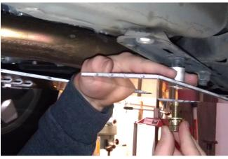
d) Grab one long bolt and washer, then put both long spacers into place on the top of the plate to where they will go up into the sub-frame, the bolt w/ washer will go up through the plate, spacer and sub-frame. Thread the nut onto the exposed threads of the bolt. Poking out of the sub-frame just underneath the control arm. On the four cylinder models the drivers side will be much more easily accessed.
