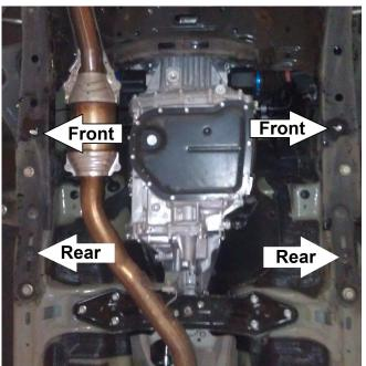
c) Determine which bolts you'll use to mount the rear of the plate: either the gold plated 7/16" or the slightly smaller silver M10. Place the shorter spacers on top of the plate where the rear mounting slots are. Lift the plate up so the spacers go around the threaded sleeves coming down off the sub-frame support bracket and thread in the appropriate bolts each with a flat washer. Leave the bolts loose and let the front of the plate hang.
