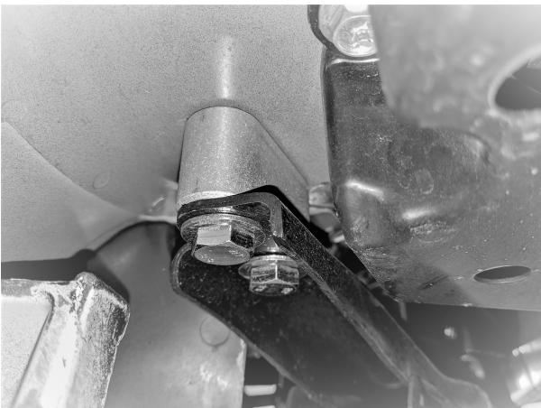
Installed forward support bracket:
