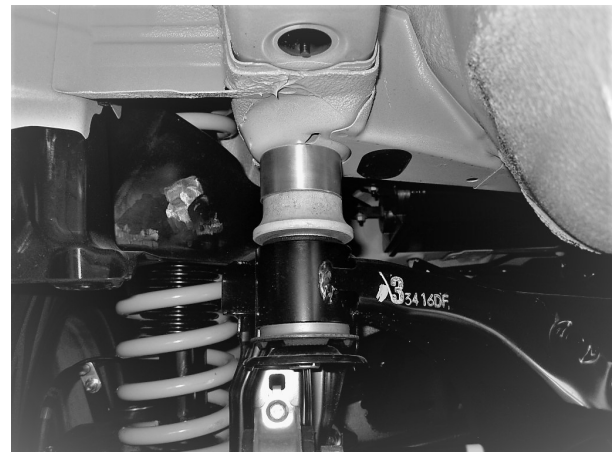
Installed subframe spacers:
