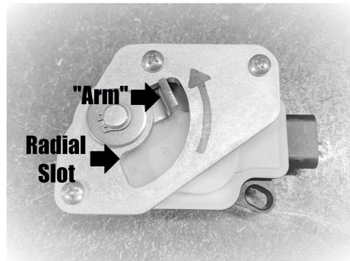
Step 6. Now that the motor is in the correct position, place a nylon spacer in between the motor and the ASE at each screw position and install the #8 screws through all three components and secure with the Nyloc nuts, use the #2 Phillips Screwdriver and the 11/32” socket to tighten everything, the torque spec for bolts this small is ~20 Inch/lbs, that's \*\*\*\*\*INCH POUNDS\*\*\*\*\* not ft/lbs, over tightening may break the mounting holes on the motor.
